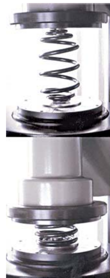
Fig. 2 — A minibloc spring unloaded (top) and loaded (bottom).
